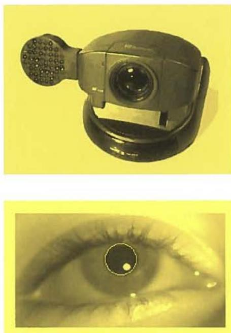
The gaze camera has to be tilted and panned to keep the eye being tracked at the centre of the image if there are head
