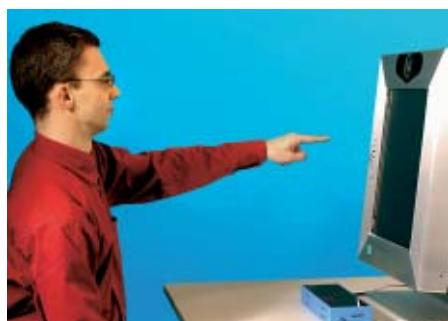
Fig. 1: The Free2C 3D display uses the head tracker to optically address the user's left and right eye. The hand tracker allows natural interaction with virtual objects floating in front of the screen.
