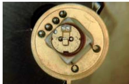
Fig. 2: DFB Laser mounted on a compact TO8 module with integrated TE cooler
