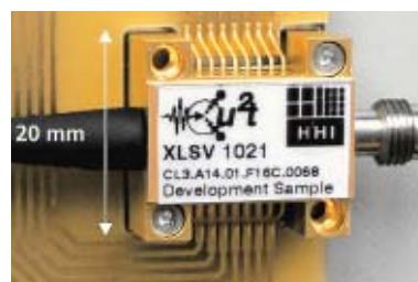
Fig. 2: Photo of the 40 GHz pulse source module
