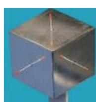
MIMO cube antenna used for channel measurements
