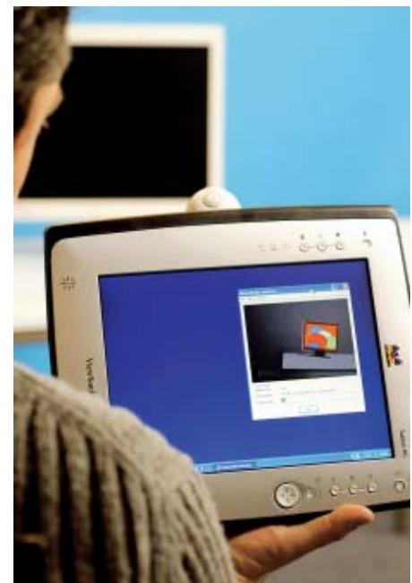
Fig. 3: The object tracker camera on top of the tablet PC captures the real scene. The software is recognizing the position and orientation of a known object (in this example an LCD monitor) and correctly matching a virtual texture. All processing is done with a simple webcam in realtime. The user can freely move the tablet PC.
