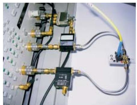
Fig. 2: Experimental set-up for testing VCSELs at wavelengths of 1.3 and 1.5  $\mu\text{m}$ , which are most important in telecommunications. Rightmost shown is the device under test
