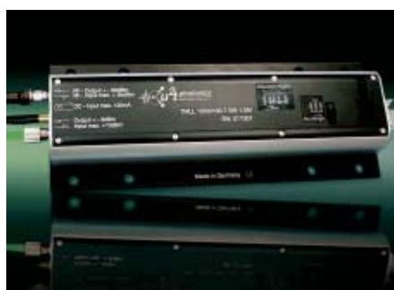
Fig. 2: Commercially available 10 GHz external cavity pulse laser source consisting of FhG-HHI's implanted 1.55µm SIPBH FP bulk laser (u2t Photonics AG, Berlin)
