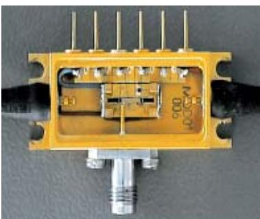
Fig. 1: Packaged MZ-Modulator for 40 Gbit/s
