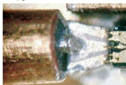
Fig. 2: 70 GHz interconnection with semi-rigid coaxial cable, CPW on alumina, and wire bonded photodiode
