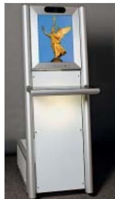
The Free2C Kiosk combines a high-resolution autostereoscopic 3D display with a gesture recognition device integrated into the panel. This novel information terminal is perfectly suited for applications in high-tech showrooms, convention halls, airports, and shopping malls
