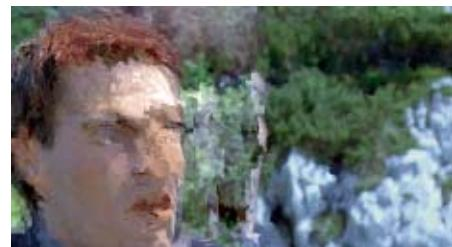
Fig. 2: Error propagation caused by video packet loss in case of variation in network capacity
