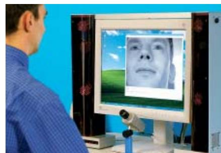
Fig. 2: Four switchable infrared spot-lights and a stationary high-resolution camera are used to measure the user's current point of fixation.
