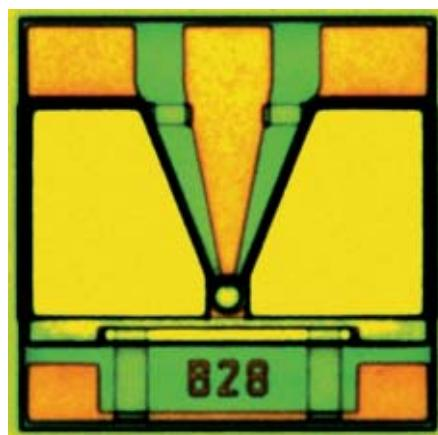
Fig. 2: Microphotograph of a 15 GHz diode with integrated termination resistor for 50 Ohm matching
