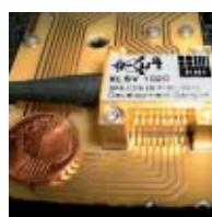
Low foot-print, packaged selfpulsating laser for clock extraction at 40 Gb/s
