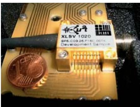
Fig. 1. Photo of a compact 40 GHz pulse laser module integrating a monolithic mode-locked laser mounted on a line-card (optical output with connected fibre on the left, electrical high frequency input port on the right, module fabrication: u2t Photonics AG, Berlin)
