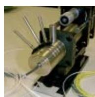
Continuously variable delay line for optical signal processing (loss variation < 0,2 dB)
