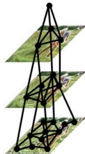
Fig. 3: Graph representation of a hierarchically segmented image (hierarchy with 3 levels of detail)
