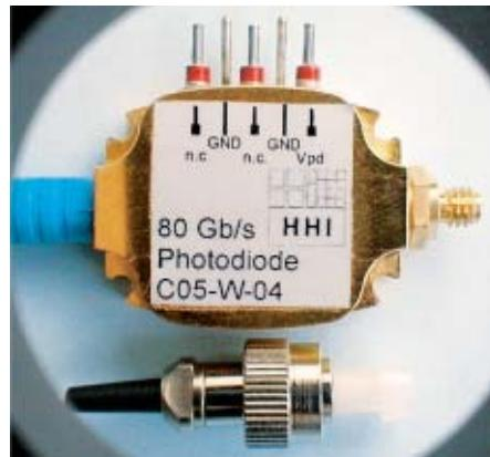
Fig. 1: 80 Gbit/s photodetector module with fibre pigtail and 110 GHz RF connector
