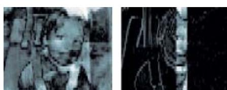
Fig. 3: Difference images between adjacent frames during a hard cut (left) and a wipe (right) used in the shot detection algorithm
