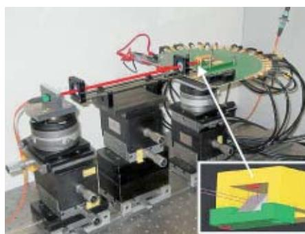
Fig. 2: Photography of the free-space optical transmission system using a 12-channel transmitter and receiver
