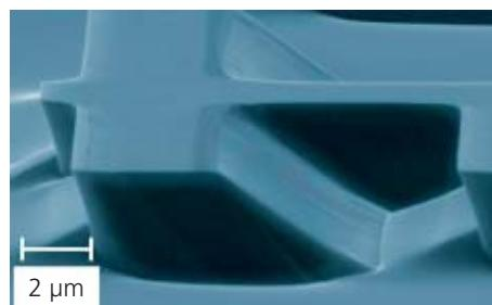
Fig. 3: Sloped sidewalls formed in InP by physical ion beam etching
