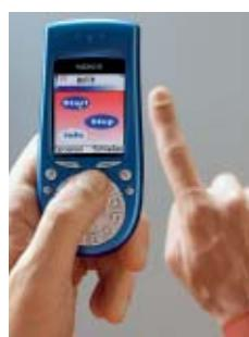
The FingerMouse uses the camera on the rear side of a mobile phone. The position of the finger tip is translated into a cursor position on the screen. For clicking the user may press a suitable button with the thumb.
