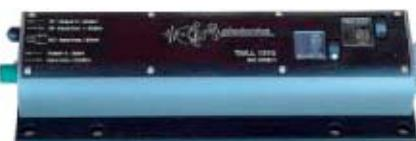
Fig. 2: Commercially available 10 GHz external cavity pulse laser source consisting of FhG-HHI's implanted 1.31 µm SIPBH FP bulk laser ("TM11310", u2t Photonics AG, [www.u2t.de](http://www.u2t.de))
