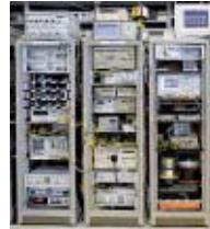
Optical loop test bed for investigation and development of S-, C-, L-band wavelength division multiplex systems with transmission rates up to 40 Gb/s per channel
