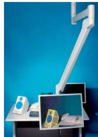
Fig. 2: The object tracker camera on top of the monitor captures the real scene. The software is recognizing the position and orientation of a known object (in this example a loudspeaker) and correctly matching the edges and a virtual texture. All processing is done in realtime. The user can freely move the articulated monitor.
