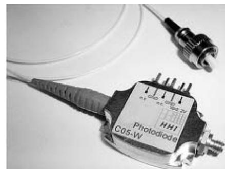
Fig. 2: Photograph of the PD module with fibre pigtail and 1 mm output connector
