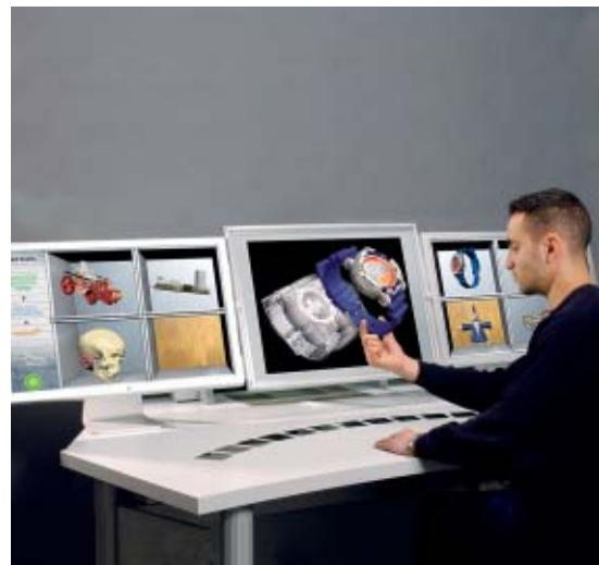
Interactive workplace allowing users to "drag" computer-generated or scanned 3D objects from the two flanking LCD displays and "drop" them into the central 3D display for direct manipulation. The video-based device for hand-gesture recognition is embedded in the desktop. The high-resolution 3D display ( $2 \times 1600 \times 1200$  RGB pixel) creates a floating 3D image hovering over the desk.
