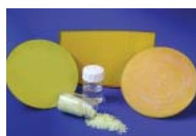
Polymer substrates and waveguide materials – The basis of low-cost photonic devices.
