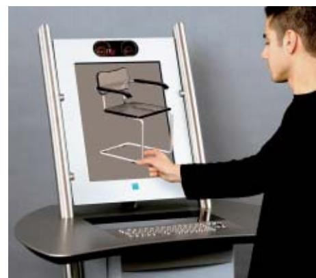
Fig. 2: The Free2C Kiosk combines innovative 3D display and gesture recognition technologies with elegant terminal design
