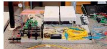
Laboratory setup of a phase stabilized optical data multiplexer
