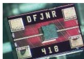
InP-Based photonic device flip-chip bonded to 100 GHz microstrip line on multilayer thin film carrier (developed in cooperation with Fraunhofer IZM).
