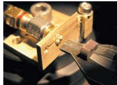
Fig. 4: Photodiode directly mounted on a V-type connector (here shown in a measurement set-up with a fibre)
